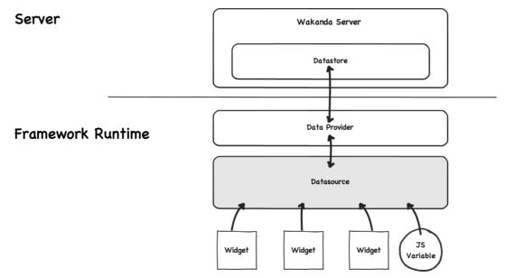
Wakanda's data provider communicates directly with the datastore on the server, typically via JSON and REST, assisted by JavaScript. The data provider handles the local cache and the parsing of data on the client, loading only the necessary data into memory. The Wakanda Doc Center discusses how to configure and use Wakanda's JSON-RPC services (see **Using JSON-RPC Services**).
